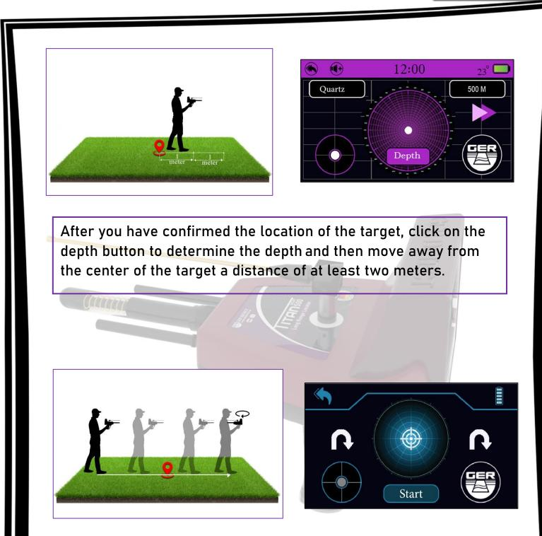
Point the device towards the target while maintaining the balance of the device, press the start button, wait until you hear a beep from the device, then walk towards the target until the device rotates backwards with the appearance of an icon indicating the rotation of the device towards the back.
