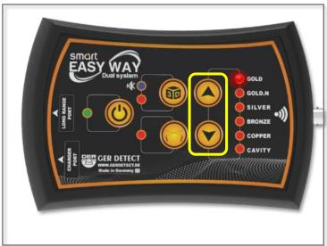
After selecting the target to be searched for, securely place the main unit to your waist and then hold the sensor grip at a **90-degree** angle in order for the antenna to function properly.
